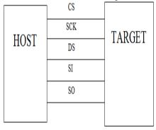
Fig. 3. Extended SPI approach
