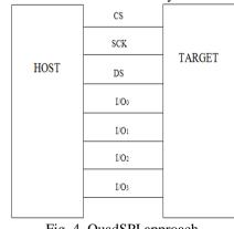
Fig. 4. QuadSPI approach
